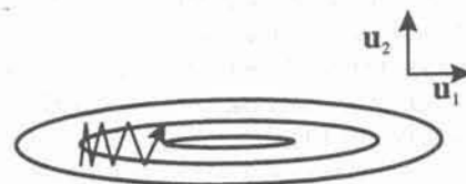
Figure 7.7. Illustration of the effect of adding a momentum term to the gradient descent algorithm, showing the more rapid progress along the valley of the error function, compared with the unmodified gradient descent shown in Figure 7.4.
